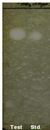
Fig. (1): A scanned image of TLC plate of the developed crude surfactin extract produced by Bacillus subtilis isolate BS5. The sample (Test) was developed against a standard (Std.) surfactin (Fluka, obtained from Sigma-Aldrich, Germany) using CHCl 3 :CH 3 OH:H 2 O at 65:25:4 v/v/v as a mobile phase.
