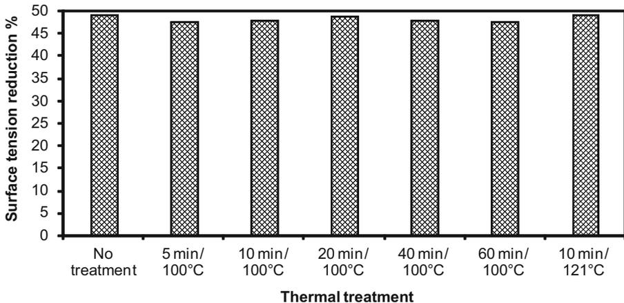
**Fig. 4** Effect of temperature on surface activity of test rhamnolipid (50 mg/l in 0.1 M sodium phosphate buffer, pH 7.2). Surface activity was expressed in terms of percentage reduction in surface tension
