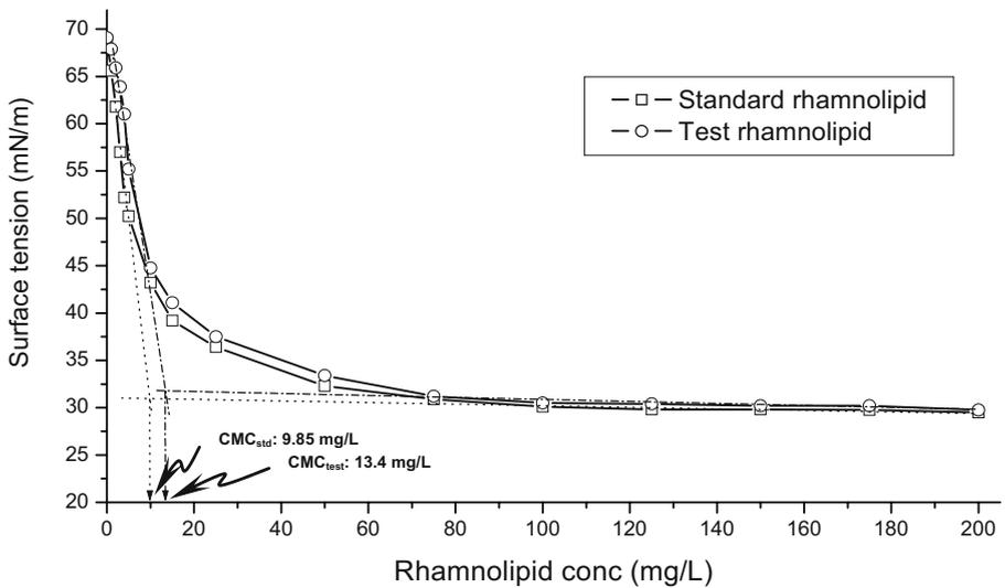
**Fig. 2** A plot of surface tension as a function of concentration of standard and test rhamnolipid at pH 7.2 in 0.1 M Na<sub>2</sub>PO<sub>4</sub> buffer
