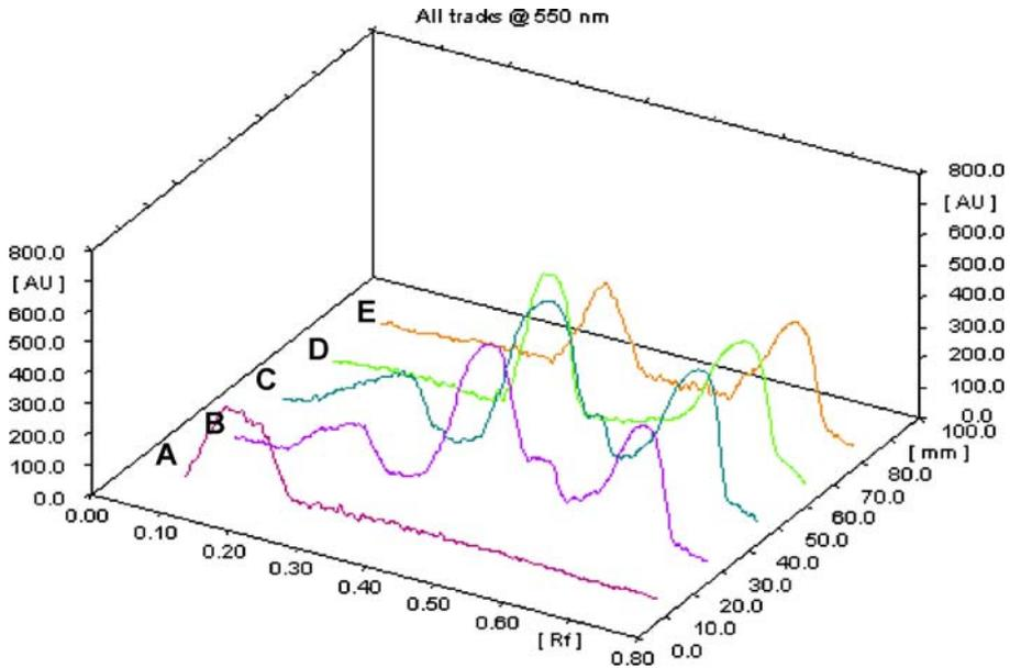
**Fig. 9** 3-D absorbance chromatograms measured at 550 nm for the different tracks obtained in Fig. 8. These chromatograms were developed using winCATS Planar Chromatography Manager software
